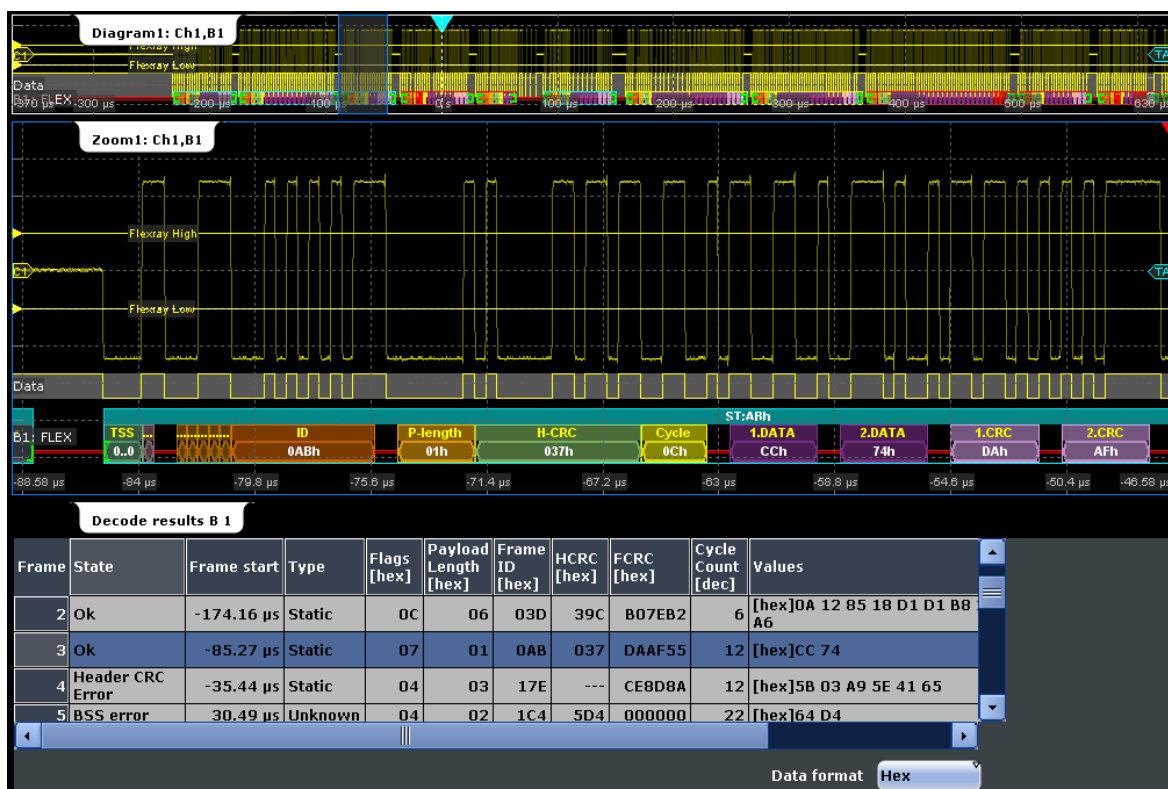
Figure 13-35: FlexRay - decoded dynamic slot and results table
